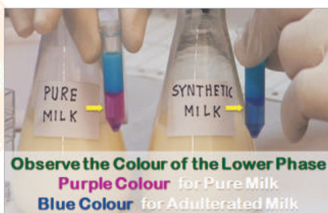
Qualitative test for detection of detergent in milk
