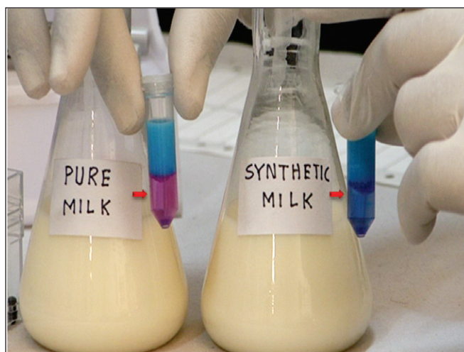
Rapid method for the detection of detergent in milk. Purple colour in lower layer indicates pure milk; blue colour in lower layer indicates presence of detergent in milk.
