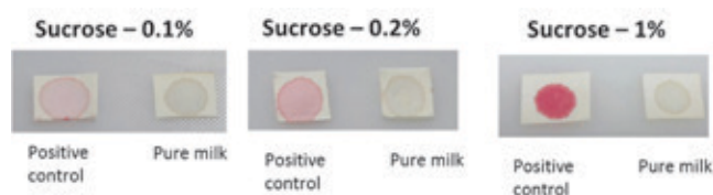
Figure: Working of the strip based test for detection of sucrose (at various levels) in milk
